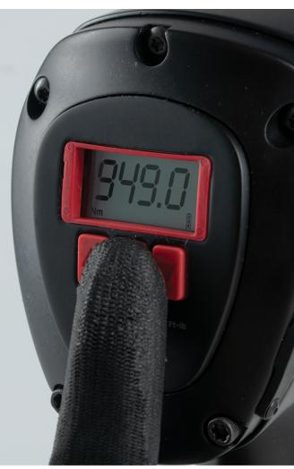
The torque value is shown on the digital display. Press the right button to toggle between units of ft-lbs (pictured above left), and Nm (pictured above right).
