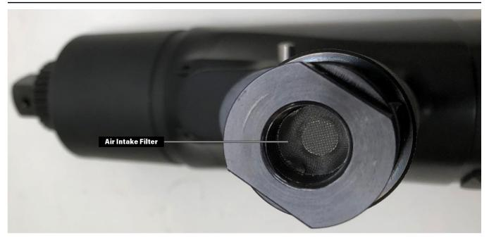
A steady, unobstructed flow of air is critical for proper performance of the **jGun DIGITAL Single Speed** Tool. The filter in the regulator intake should be cleaned frequently. In heavy use applications this filter may need to be cleaned every day. Apply forced air to unclog and clean the filter for most applications.
