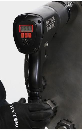
Once the trigger is pulled, the tool freezes the screen and displays the target torque applied. This screen freeze remains in effect until released. To release (un-freeze) the screen press and hold the left button for 3 seconds until the screen flashes once, then adjust the regulator (at least +/- 10% of the previous value). This screen freeze occurs for both tightening and loosening operations.
