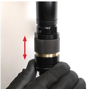
The torque value is shown on the digital display. The torque can be increased and decreased by turning the pressure regulator.
