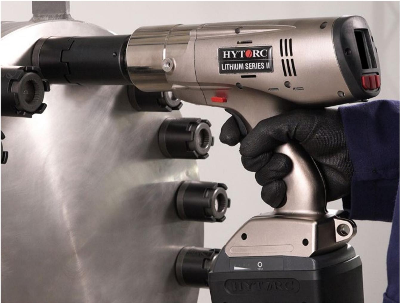
NOTE: The HYTORC Nut inner sleeve is tightened in the counter clockwise direction (left hand threads).
