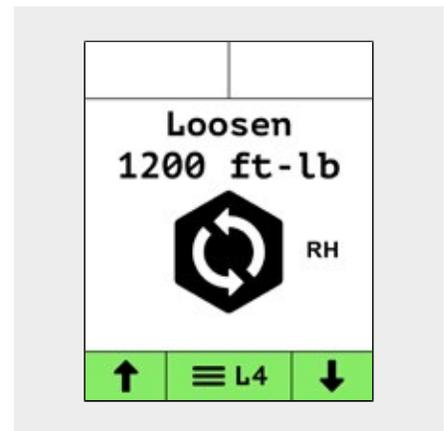
The example shows the change in direction for right hand (RH) fasteners. The directional control switch automatically sets the appropriate direction for left hand fasteners, HYTORC Washers and for the HYTORC Nut as well.
