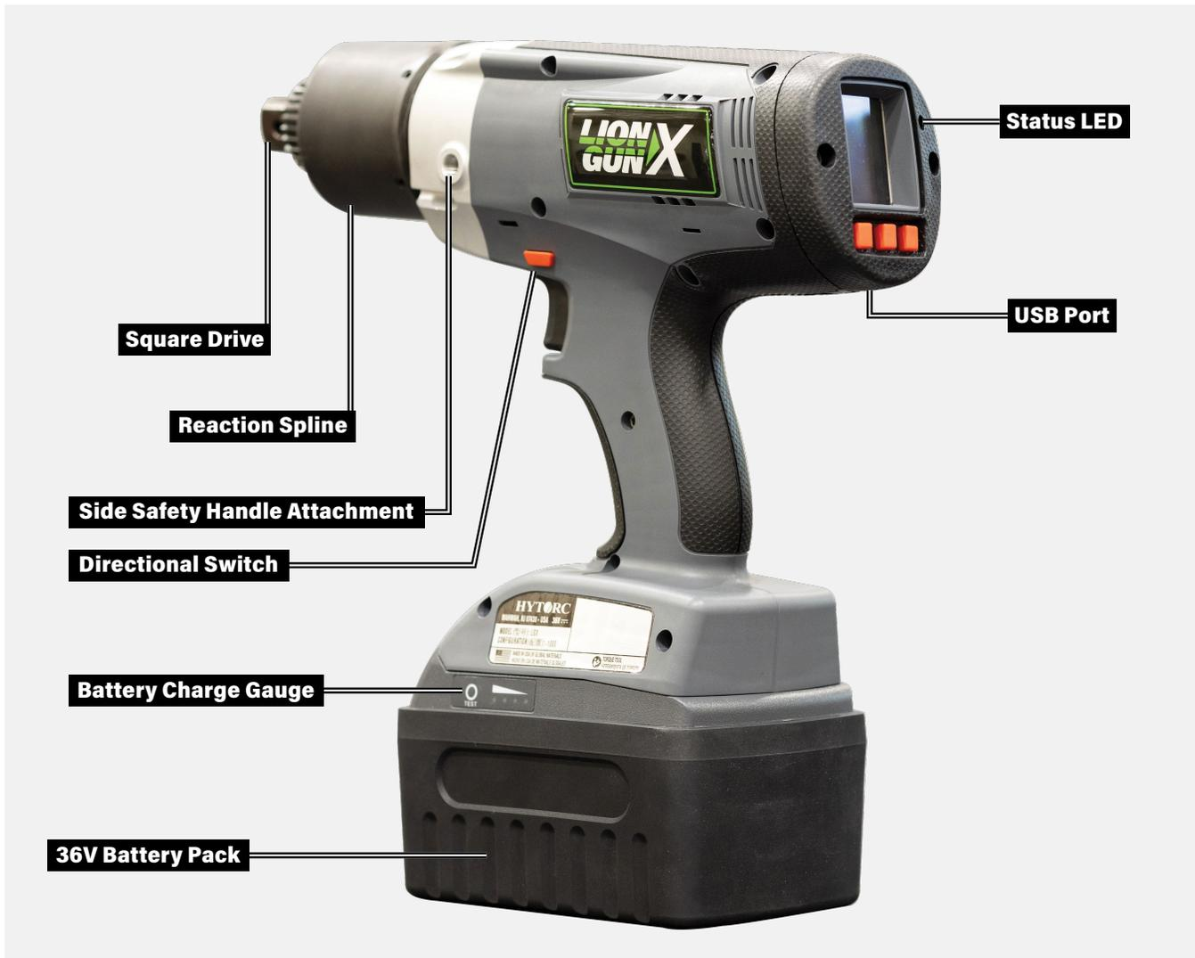
The **LION GUN® X** Electric Torque Tool has built-in data recording, a torque capacity of up to 3,000 ft.-lbs. (4067 Nm) and is powered by a 36V high-density battery pack. Users can record jobs via Bluetooth or USB cable. This tool is compatible with conventional sockets with reaction arms, the HYTORC Washer and the HYTORC Nut.
