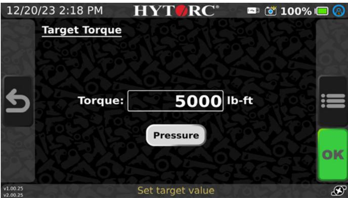
**The "Pressure" button is not provided to input data for this purpose. The pressure is only entered for service purposes or if no pressure/ torque chart is available from the manufacturer.**
