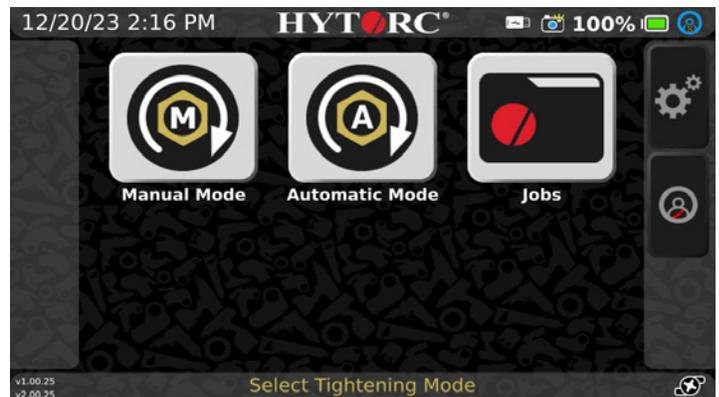
The start screen appears after switching on the pump.
