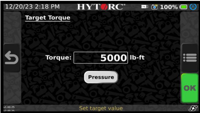
The target torque is displayed.
