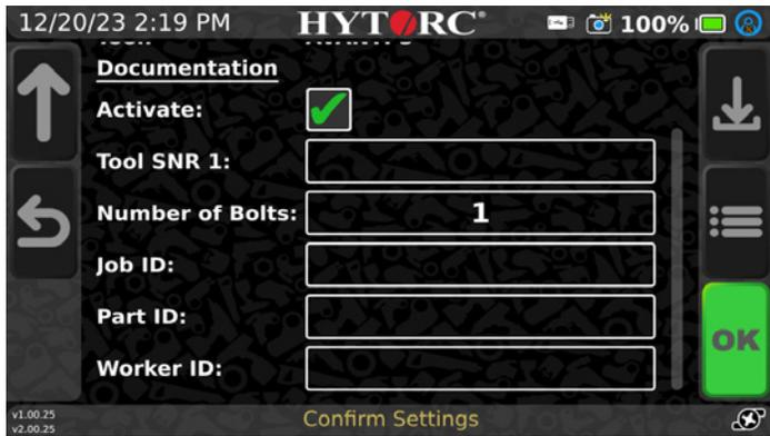
Example: Number of bolts - This is where you specify how many bolting operations you want to carry out in one process. If more than one bolting operation is involved, you will be prompted to move to the next step during the bolting process.
