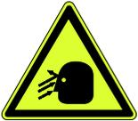
Risk of eye damage due to splashing liquid
