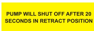
The unit switches itself off automatically after 20 seconds in the return stroke position.
